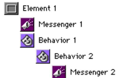
To illustrate, in the figure above, Element 1 is the parent of Behavior 1 and Messenger 1, and Behavior 1 is the parent of Behavior 2 and Messenger 2. Both messengers and behaviors are, however, associated with Element 1,
