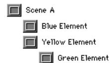
Note that the Green Element in the previous diagram is indented relative to the Yellow Element, indicating their new parent/child relationship. Parent/child relationships can also be made in the layout window using the Parent/Child Tool (see “Parent/Child Tool” on page 11.106).
