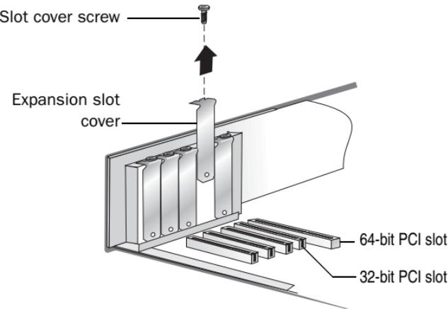
5 Insert the DuoConnect adapter in the PCI expansion slot. Press the adapter firmly into the slot until it clicks into place. Replace the slot cover screw. When installed properly, the adapter should be level with the expansion slot, as shown below.
