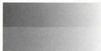
The lower bar shows the shift away from black when the black point is too low.
