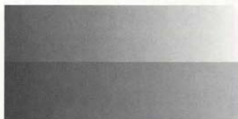
The lower bar shows the shift to gray when the white point is too low.
