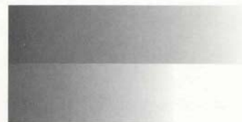
The lower bar shows the shift to white when the white point is too high.
