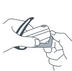
1 Remove the top strap and unseat the SDM pod from the bottom clip.
