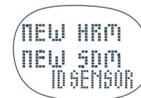
**NOTE:** Once you have linked the SDM pod for the first time, the watch will remember the digital ID until you switch to a different pod. If you would now exit PC mode and re-enter ID SENSOR LINKING, the display would read SDM instead of NEW SDM.
