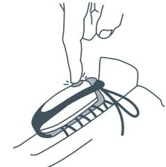
4 Turn SDM pod ON. Press and hold power button until LED light begins to blink.
