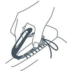
3 Secure the SDM pod with black strap. The pod should rest just below where laces tie and be secure enough to stay in place during workout.
