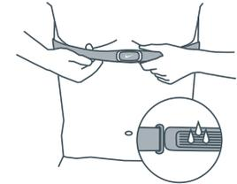
4 Generously wet both sensors on the back of the HRM transmitter to ensure strong connection between your pulse and the transmitter.
