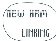
**NOTE:** Once you have linked the HRM transmitter for the first time, the watch will remember the digital ID until you switch to a different transmitter. If you would now exit PC mode and re-enter ID SENSOR LINKING, the display would read HRM instead of NEW HRM.
