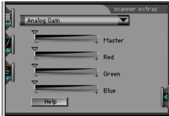
Moving a slider to the right increases the intensity of the affected LED; moving it to the left decreases the intensity. Click the **Help** button for information on using analog gain.
