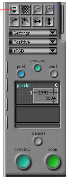
If the optional SF-200 slide-feeder is inserted in the LS-2000, clicking the eject button ejects the current slide and feeds the next slide from the feed magazine.
