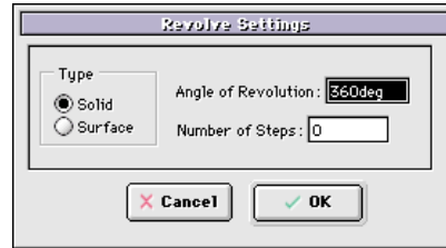
Figure 2.23 — Revolve tool settings
