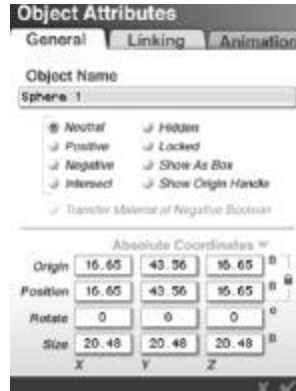
The Object Attributes dialog contains controls for setting the object's name, scale, position, and orientation.
