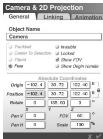
The Camera & 2D Projection dialog lets you view and set the attributes of the current camera.
