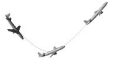
If you align the airplane to its path, the airplane's nose tilts down as it moves down and up as it moves up.
