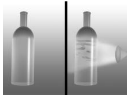
The Light Sensitive mode was used to apply material inside the bottle on the left. When the bottle is lit by a light source, the particles of the material become visible creating the effect of a light beam passing through the bottle.
