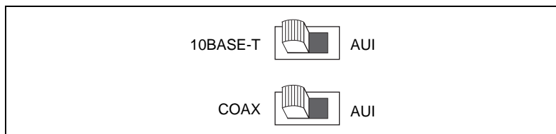
Figure 2-2. Default Ethernet Port Configuration Switch Setting for Either Type of GPIB-ENET
