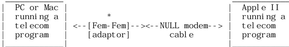
One possible disadvantage of this method is that signal lines may be missing and you will not be able to get hardware handshaking. (Tests using the IW-I cable on a IIgs showed no loss of speed under Spectrum or ADTgs.)
