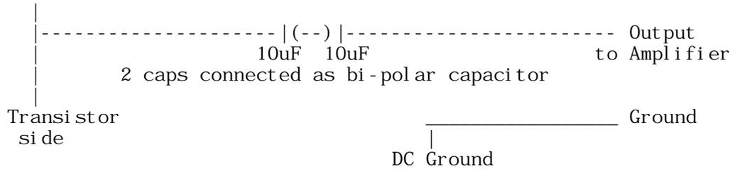
You can get a bi-polar coupling capacitor at Radio Shack or make one by connecting two 10uF caps neg end to neg end. The value is not critical, a 2uF-5uF bipolar cap or two 5uF caps connected back to back is fine. Voltage rating should be 10V or better.
