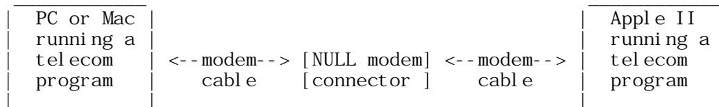
"NULL modem" means "no modem". A NULL modem connector is just a pair of connectors wired 'back to back' with a few lines switched so that each computer views the other pretty much as though it were a modem. Radio Shack, Marlin P. Jones, and other places sell NULL modem adaptors in the form of small modules or short cables for a few dollars; or, you can make your own.
