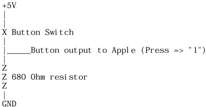
As shown below, a PC stick button Output is normally an unconnected wire. Most likely, inside the computer, a PC or compatible Game Port has this line tied to a 1k-3k resistor going to +5V. So, the line will normally be at something close to +5V (= logic 1). Pressing the button grounds the line and pulls it down near to 0V (= logic 0).
